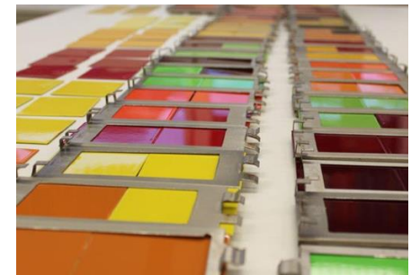
Coating testing/Anti corrosion
